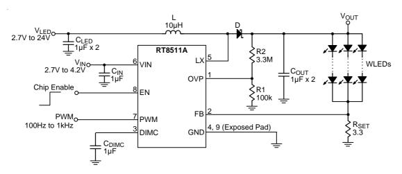
Figure 2. Typical Application Circuit of Low Voltage Operation
