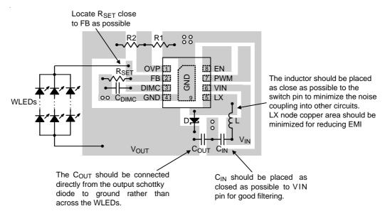
Figure 7. PCB Layout Guide
