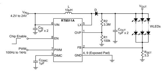
Figure 1. Typical Application Circuit of Normal Operation
