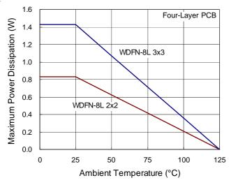
Figure 6. Derating Curve of Maximum Power Dissipation
