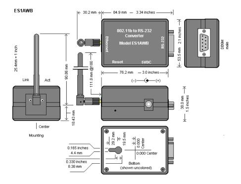
Figure 17. Dimensional Diagram of the ES1AWB
