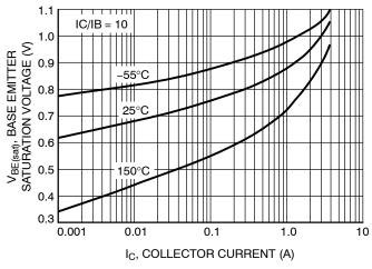
Figure 4. Base Emitter Saturation Voltage vs.
