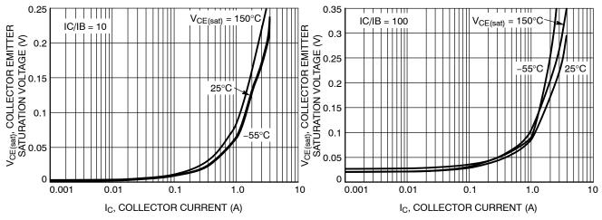
Figure 1. Collector Emitter Saturation Voltage vs. Collector Current
