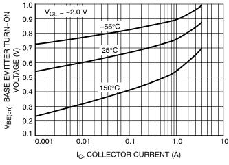
Figure 5. Base Emitter Turn-On Voltage vs.
