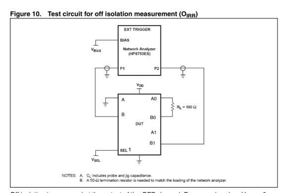
Off isolation is measured at the output of the OFF channel. For example, when  $V_{SEL1}=0$ , and B is the input, the output is measured at B1. All unused analog input ports are connected to GND and output ports are left open.
