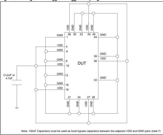
Diagram for suggested  $V_{\mbox{\scriptsize DD}}$  decoupling Figure 3.
