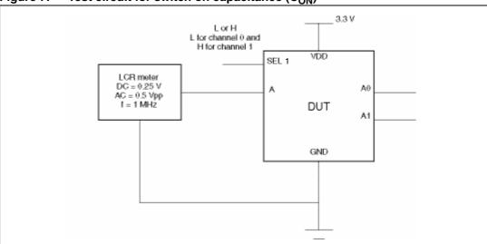
Figure 7. Test circuit for switch on capacitance (C<sub>ON</sub>)
