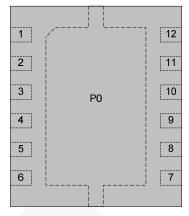
Figure 3. 12-Lead MLP (Top View)
