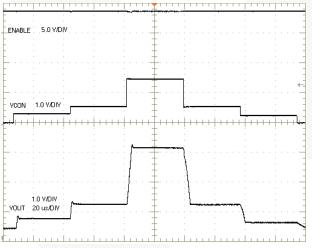
Figure 7. Rise Times for 300mV, 500mV, and 2V  $\Delta V_{OUT}$   $C_{OUT}$  = 2.2µF (V<sub>IN</sub>=3.7V)
