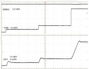
Figure 8. Rise Times for 300mV, 500mV, and 2V  $\Delta V_{OUT}$  C<sub>OUT</sub> = 2.2 $\mu$ F (V<sub>IN</sub>=3.7V)
