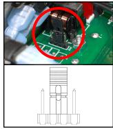
Figure 5. 110V jumper setting
