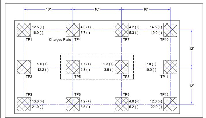
Figure 7. 50664 Neutralization (Discharge) Times at 100VAC, 50Hz input
