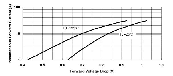
Fig.3-Typical Instantaneous Forward Voltage Characteristics
