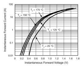
Fig. 3 - Typical Instantaneous Forward Characteristics
