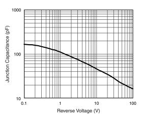
Fig. 5 - Typical Junction Capacitance
