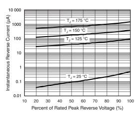
Fig. 4 - Typical Reverse Characteristics
