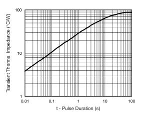
Fig. 6 - Typical Transient Thermal
