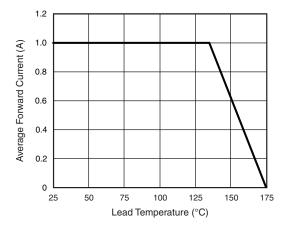
Fig. 1 - Forward Current Derating Curve
