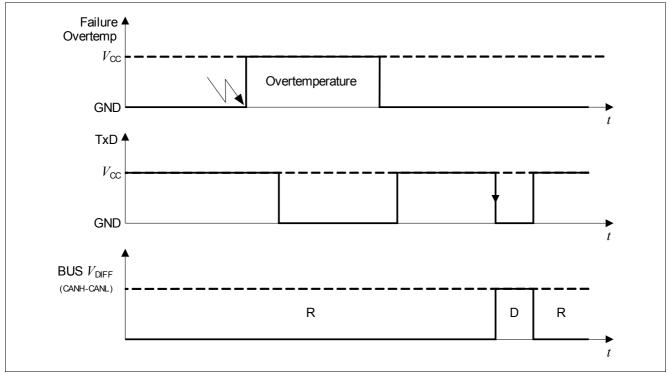
Figure 4 Release of the Transmission after Overtemperature
