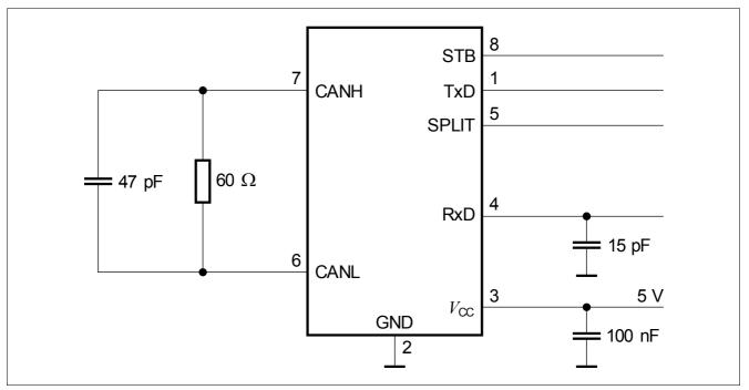
Figure 8 Test Circuit for Dynamic Characteristics
