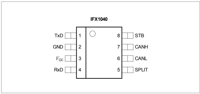
Figure 1 Pin Configuration IFX1040SJ (top view)
