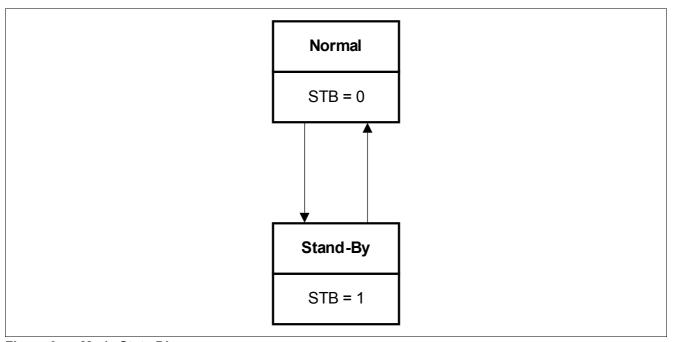
Figure 3 Mode State Diagram
