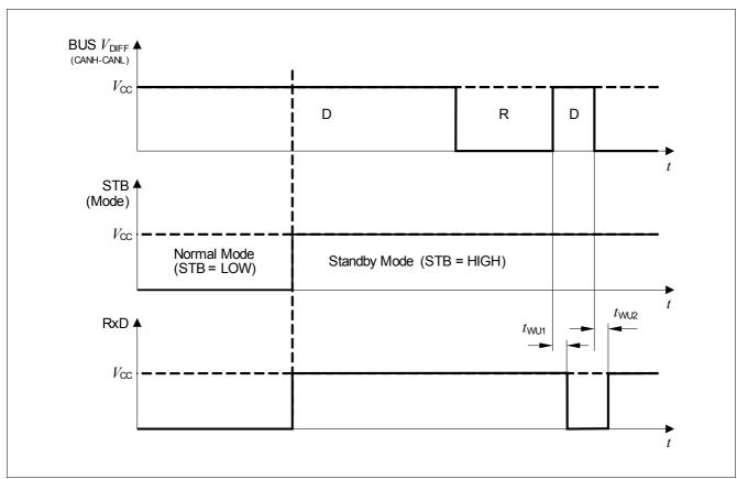
Figure 5 Go-To Standby Mode during Bus Dominant Condition
