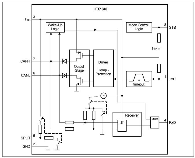
Figure 2 Block Diagram IFX1040SJ
