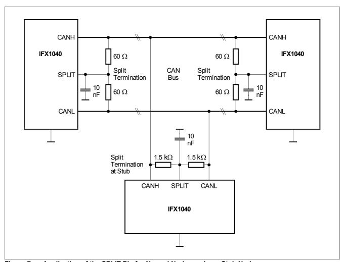
Figure 7 Application of the SPLIT Pin for Normal Nodes and one Stub Node
