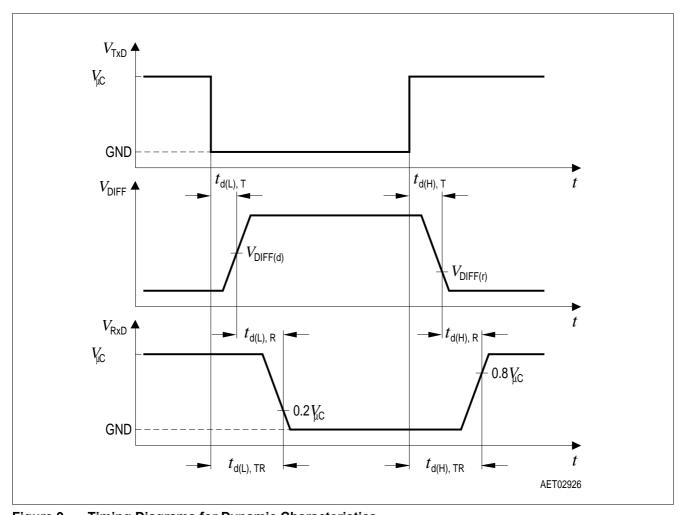
Figure 9 Timing Diagrams for Dynamic Characteristics
