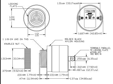
NOTE A: TERMINALS-032 BRASS TIN PLATED, TAPPED FOR #6-32 SCREW. TWO #6-32 NICKEL PLATED BRASS SCREWS INCLUBED. WILL ACCEPT 1/4' QUICK CONNECT. NOTE B: MOUNTING- REMOVE BLACK PLASTIC NUT AND INSERT THREADED FRONT THROUGH 1.25' HOLE PUNCHED IN PANEL, IF DRIENTATION IS NEEDED, NOTE LOCKING FLATS ON DRAVING. SCREW NUT BACK ON. DO NOT DVERTIGHTEN.
