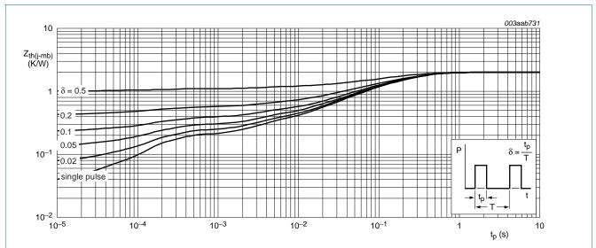
Fig 4. Transient thermal impedance from junction to solder point as a function of pulse duration
