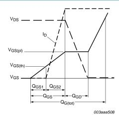
Fig 10. Gate charge waveform definitions
