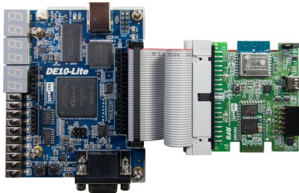
Figure 4-7 Setup ESP8266 Web Server Demo
