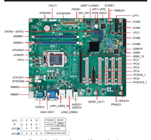
Figure 1: Board Layout: Jumper and Connector Locations
